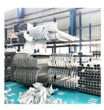
The frame profile is designed and manufactured by the national standard 140\*140\*4 square tube. The surface is hot-dip galvanized, the finished product is assembled, the screws are all 8.8 grades, no on-site welding is required, and the service life is more than ten years.
