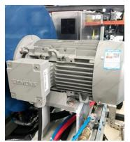
The main power motor and the air-drying system motor all adopt the imported aluminum shell motor from Siemens Germany, which has lower energy consumption and longer service life.
