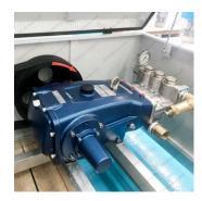
Stainless steel pump head, aluminum alloy crankcase, German imported sealing ring, more than ten years of service life.
