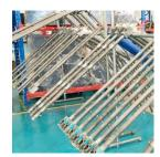
Full 304 stainless steel double-side spray rod ensures that pipes and lifting devices are not rusty.
