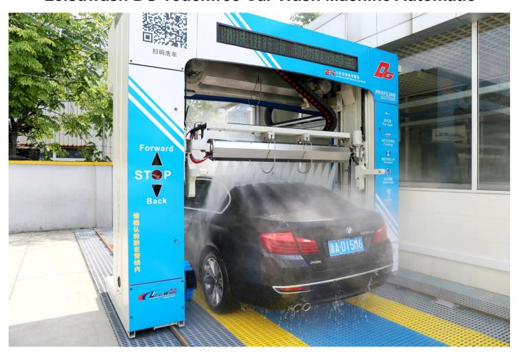
Washing without brushes poses a special challenge for a car wash. Leisuwash DG equipped a multi-stage chemical and high-pressure system. Automatically detect various types of vehicles and working with 35cm flushing distance and 100bar flushing pressure.
