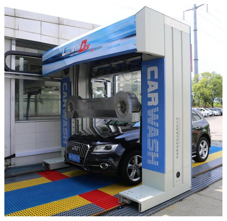
Following the Leisuwash philosophy there is no great car wash without a great drying system. Leisuwash DG flow-optimized drying system provide contour-following air drying with accurately drying distance at 25cm.
