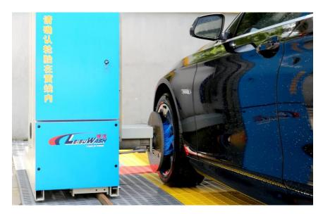
One of the most difficult areas of vehicles to clean are the wheels, Leisuwash DG takes tire scrubbing to a new level. During the process, each tire receives a chemical application and the wheel receives an intense bi-directional rotational scrubbing, combined with high-pressure water flow. There are multiple cleaning technologies in play to meet even the most demanding consumer needs.
