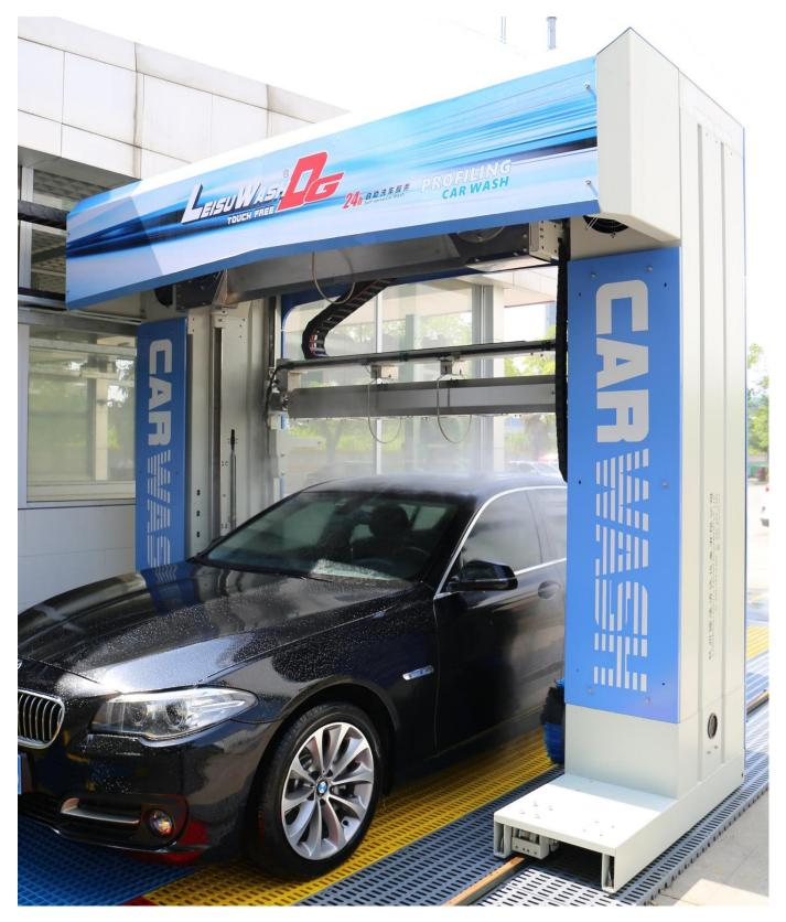
A multi-stage applicator is used to apply different chemicals and therefore loosens a high amount of dirt. Contour-following and lateral high pressure ensure that the vehicle surface is cleaned thoroughly after the dirt has been loosened.
